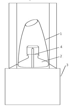
The lamp cartridges (2) are replaceable. Follow the diagram above to replace the cartridge.
